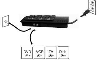
Connect the coaxial cable from your cable / antenna / dish source to one of the surge protector's video connectors marked "IN". With another section of coaxial cable, connect the surge protector's corresponding video connector marked "OUT" to the appropriate jack on your tv/vcr/other device.
