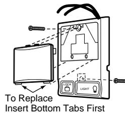
**Figure 2** PRE-WIRED INSTALLATION
