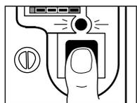
2. Within 30 seconds, press and hold the button on the hand-held remote\* that you wish to operate your garage door.
