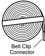
3. Fasten the belt clip connector to the trolley clip with a master link:
