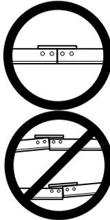
Improper assembly can cause jerky trolley operation, noise and/or nuisance door reversals.
