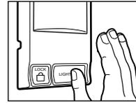
3. Continue holding both buttons while you press the push bar on the Multi-Function Door Control (all three buttons are held).
