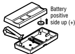
Dispose of old battery properly. Replace the battery with only 3V2032 coin cell batteries.
