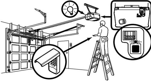
1. Press and release the "learn" button on motor unit. The learn indicator light will glow steadily for 30 seconds.
