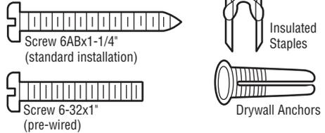
**Figure 1** PRE-WIRED INSTALLATION
