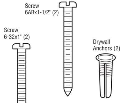
**NOTE:** For gang box installations it is not necessary to drill holes or install the drywall anchors. Use the existing holes in the gang box.
