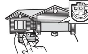
The garage door opener will not close from a remote control if the LED in either safety reversing sensor is off (alerting you to the fact that the sensor is misaligned or obstructed).
