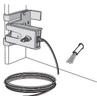
**2.2B** Separate the safety reversing sensor wires and strip 7/16 inch (11 mm) of insulation from each end. Choose two of the pre-installed wires and strip 7/16 inch (11 mm) of insulation from each end. Make sure that you choose the same color pre-installed wires for each sensor.
