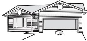
**3.2** Press the remote control push button to close the door. The door will not move more than an inch (2.5 cm), and the garage door opener lights will flash 10 times.
