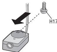
**1.4C** Insert the bolt through the hole in the sensor bracket and attach with the wing nut (H18). The lenses on both sensors should point toward each other. Make sure the lens is not obstructed by the sensor bracket.
