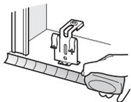
**1.2C** Attach the sensor brackets to the floor using concrete anchors (not provided).
