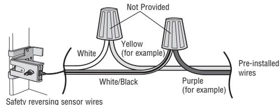
**2.4B** At the garage door opener, strip 7/16 inch (11 mm) of insulation from each end of the wires previously chosen for the safety reversing sensors. Twist the like-colored wires together.
