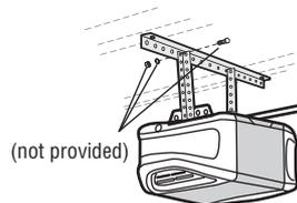
**5.5** Attach the garage door opener to the hanging brackets with the bolts (H21), lock washers (H15) and nuts (H20).
