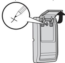
**1.7** Remove the door control from the wall and drill a 5/32 inch (4 mm) hole for the top screw.
