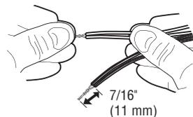
**2.3A** Insert the white wires into the white terminal on the garage door opener. Insert the white/black wires into the grey terminal on the garage door opener. To insert or remove the wires from the terminal, push in the tab with a screwdriver tip.
