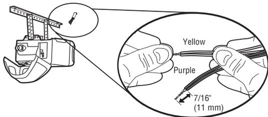
**2.5B** Insert the wires connected to the white safety sensor wires to the white terminal on the garage door opener. Insert the wires that are connected to the white/black safety sensor wires to the grey terminal on the garage door opener.
