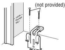
**1.3C** Slide the carriage bolt (H17) into the slot on each sensor.
