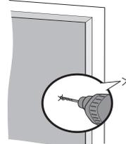
**1.8** Position the bottom hole of the door control over the screw and slide down into place. Attach the top screw.
