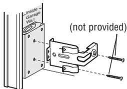
**1.3B** Slide the carriage bolt (H17) into the slot on each sensor.
