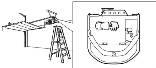
2 Press and immediately release the Learn button. The Learn LED will glow steady for 30 seconds. Within 30 seconds...
