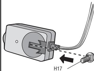
**1.3A** Insert the bolt through the hole in the sensor bracket and attach with the wing nut (H18). The lenses on both sensors should point toward each other. Make sure the lens is not obstructed by the sensor bracket.
