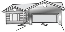
**2.2** Press the remote control push button to close the door. The door **MUST** reverse when it makes contact with the board.
