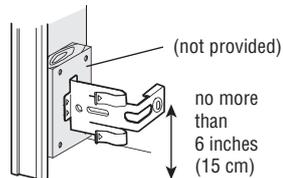
**1.2B** Drill 3/16 inch pilot holes for each sensor bracket and attach the sensor brackets to the wall using lag screws (not provided).
