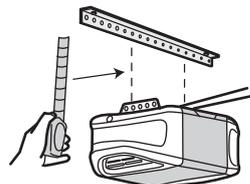
**5.3** Cut both pieces of the hanging bracket (not provided) to required lengths.
