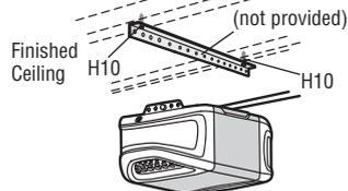
**5.2** Make sure the garage door opener is aligned with the header bracket. Measure the distance from each side of the garage door opener to the support bracket.
