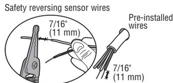
**2.3B** Connect the pre-installed wires to the sensor wires with wire nuts making sure the colors correspond for each sensor. For example, the white wire would connect to the yellow wire and the white/black wire would connect to the purple wire.
