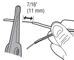
**2.3** Connect the wire to the red and white terminals on the garage door opener. To insert or release wires from the terminal, push in the tab with screwdriver tip.
