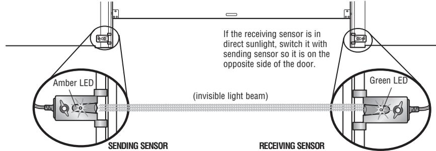
**IF THE AMBER LED ON THE SENDING SENSOR IS NOT GLOWING:**
