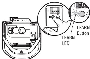
3 Press and hold the button on the remote control that you wish to use. Release the button when the garage door opener lights blink or two clicks are heard.
