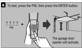
To program the Keyless Entry to more than one garage door opener, repeat the steps above using a new PIN for each additional garage door opener.
