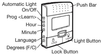
This door control contains a motion sensing detector that will automatically turn on the light when it detects a person entering the garage.
