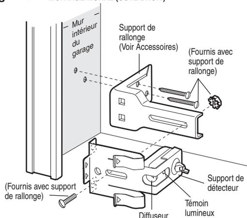
Figure 4 MONTAGE AU SOL (CÔTÉ DROIT)
