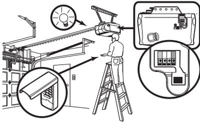
1. Press and release the “learn” button on motor unit. The learn indicator light will glow steadily for 30 seconds.
