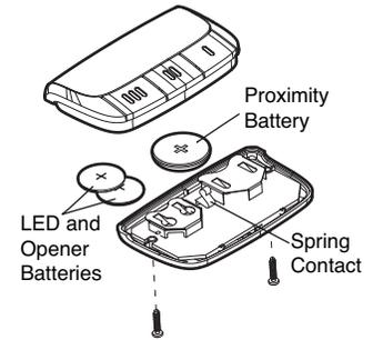
To replace the batteries, remove the two screws and open the remote control housing. Push the battery out of the holder for removal.
