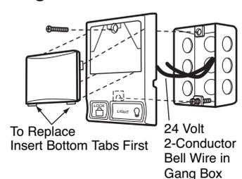
**Figure 3** MULTI-FUNCTION DOOR CONTROL (BACK)
