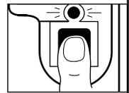
1. Press and release the “learn” button on the motor unit. The learn indicator light will glow steadily for 30 seconds.
