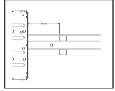
2. With chain tensioned, lift up the chain and place noise reduction pads under the chain in orientation shown.
