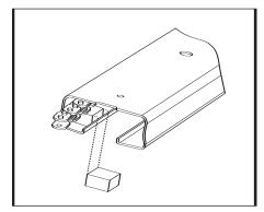
Clean and remove grease from rail in areas where pads will be installed.
