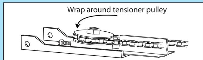
FIG. 1-4 Mount chain/belt to tensioner pulley.
