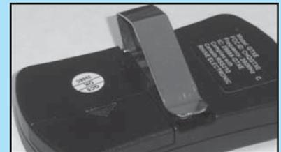
FIG. 8-3 Attach visor clip.
