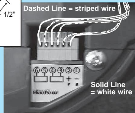
FIG. 4-8 Insert wires
