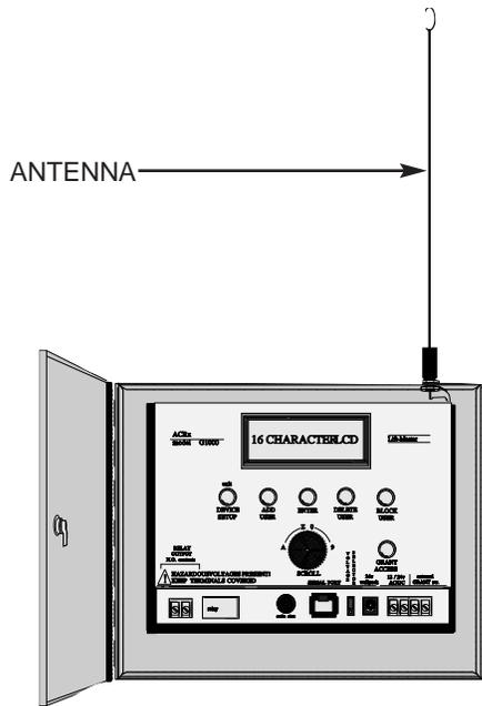
B. No amplifier, coax cable used (short radio range).
