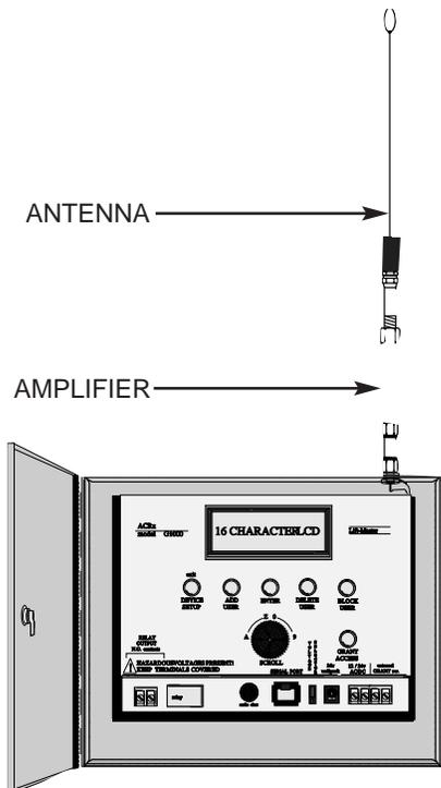
D. Amplifier and coax cable used (longer radio range).
