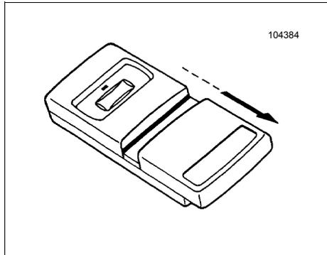
**RECEIVER:** The Receiver Coding Switches can be accessed by removing the small door from the back of the Receiver using a small screwdriver or knife.
