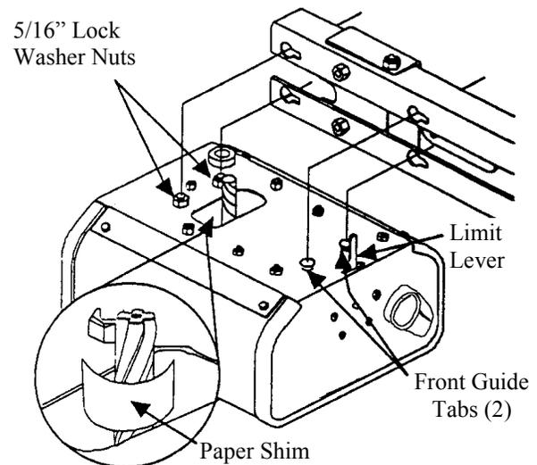
**STEP 5:** The power head drive unit should be move forward until all play between the gears has been eliminated, but no additional force should be used that could cause pressure on the motor (power head unit) drive gear. Tighten the two 5/16" lock washer nuts on top of the power head drive unit that were loosened in Step 2 above.
