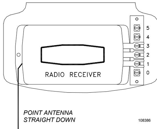
After installing the Radio Controls, check their operation by moving approximately 35 FT away from the garage door and pressing the Transmitter Button. Operation at this distance should be reliable.
