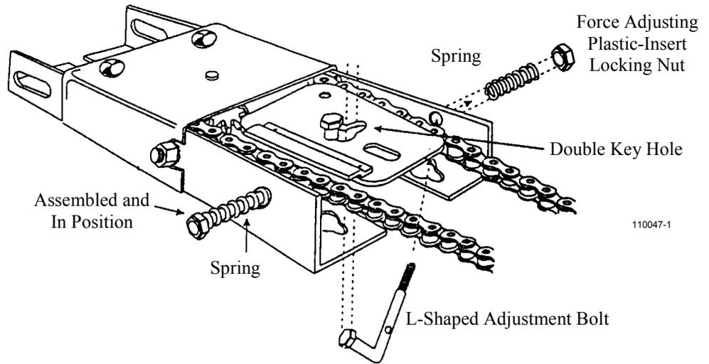
**STEP 2:** Protect the Power Unit cover from scratching during assembly by placing it on cardboard. Loosen the two 5/16" lock washer nuts on top of the power head drive unit.
