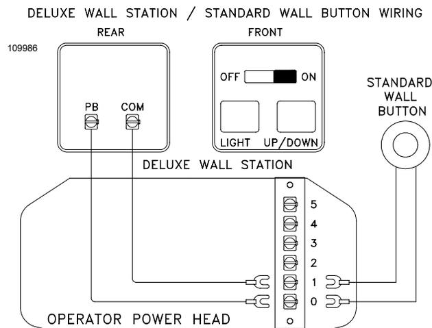
**Step 5:** Install the Control Button Warning Label supplied with your Challenger AC9000 Series operator near the control button (see illustration). Repeat the Steps 1 thru 5 above to install additional standard wall push buttons if desired. Every control must have a separate Control Button Warning Label mounted near it.
