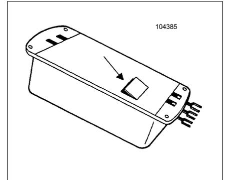
**Setting The Coding Switches:** When setting the Coding Switches THE FACTORY PRE-SET CODES MUST BE CHANGED TO PREVENT UNAUTHORIZED OPERATION. Transmitter and Receiver codes must be set IDENTICALLY. If just one Code Switch is mismatched, the Radio Controls will not function.
