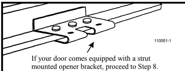
If your door comes equipped with a strut mounted opener bracket, proceed to Step 8.
