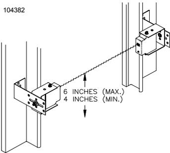
Using the 1/4” x 1-1/2” lag screw provided, attach the wall bracket securely to the wall. In some installations it may be necessary to attach wooden spacers to the wall to achieve the required clearance. Expansion bolts (not supplied) may be required to attach brackets to walls constructed of materials other than wood or gypsum. Repeat for the wall bracket on the other side of the door opening.
