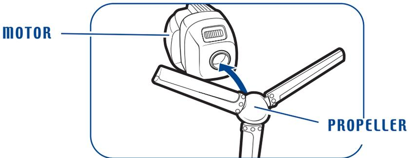
3. Properly align motors with notches in wing sockets, as shown. Motors will snap securely into place. Left side motor has white triangle.
