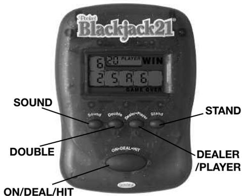
**SOUND button** - Press to turn the sound on/off.
