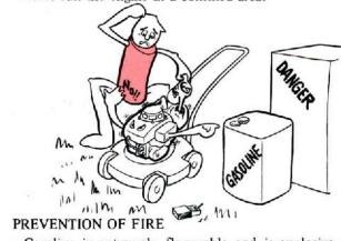
· Gasoline is extremely flammable and is explosive under certain conditions. Refuel in a well ventilated area with engine stopped. Do not smoke or allow open flames or sparks in the area where the GV35 is refueled or where gasoline is stored.
