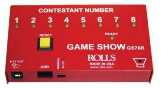
The MANUAL - AUTO switch is located on the side of the GS76R main unit. The silk-screening will indicate which selection is in use.
