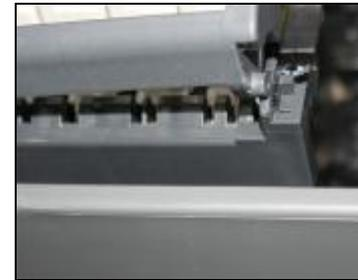
First place the left side of cartridge cover down correctly, second, put the other side of the cartridge cover at the above of the cart and adjust the position of the connection
