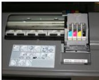
Then press the right side of the cartridge cover to make it down to the suitable position, now it is ok to work.
