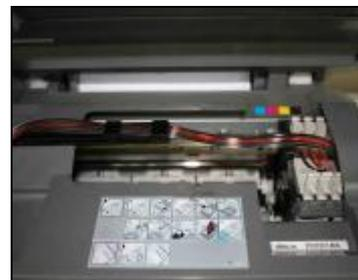
Clamp the tube on the support arm
