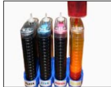
Please pay attention to the ink level in the reservoirs; if the ink level is below 1CM as the above picture shown, please use refill kits to fill ink into Reservoir bottles. Carefully pull out the rubber plugs from the refill holes.(there is possibility of ink spattering. Be careful!) Refill ink according to the color in short supply. Then put the rubber back. **(Please keep the printer and the reservoir at the same horizontal line during the process of refilling ink.)**
