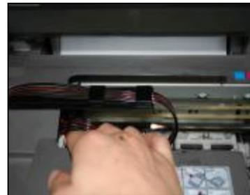
Adjust the tube length and move the cartridge car. Insure there will no block and collision when the tubes moving with cartridge car .Insure there's plenty length of tube to make the cartridge cart can thoroughly move to the left side.
