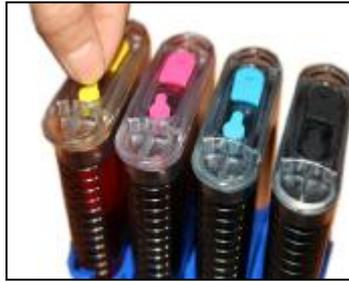
Pull out the small rubber plug from the air hole as above picture shown.
