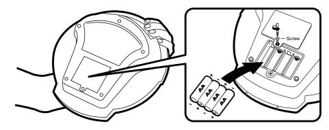
Using a Philips® screwdriver, remove the screw on the battery compartment door and remove the door.
