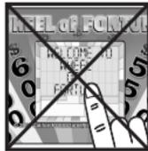
Do not press the liquid crystal display and avoid heavy shock or the display may fail.
