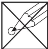
Do not use a pencil or pin to press the RESET switch. Use a ball-point pen.
