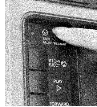
3. Press the tape pause/restart button for about 1/2 second to record the program-pause signal.
