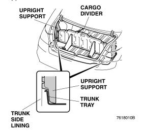
NOTE: When accessing the spare tire, remove the cargo divider and cargo nets before removing the trunk floor mat.
