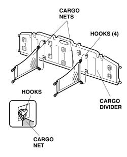
• Slide the four pins of the cargo divider into the upright support. Attach the cargo nets to the anchor on the rear trim.
