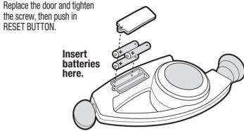
When to change the batteries: If BOP IT doesn't operate properly, or game performance changes, try reinserting the batteries. If that doesn't work, remove the old batteries, then insert three new batteries.
