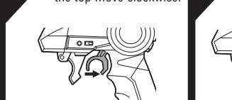
2 Move the trigger to center to make the top spin in place.
