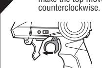
4 Press and hold the button while pushing or pulling the trigger to activate the ENGINE GEAR™\* speed burst!
