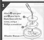
Note: Make sure screw is completely attached.
