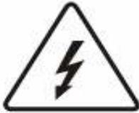
This symbol is intended to alert the user of the presence of non-insulated "dangerous voltage" within the product's enclosure that may be of sufficient magnitude to constitute a risk of electric shock to a person.
