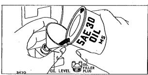
Remove the oil filler plug. Place the engine level. Fill the crankcase to overflowing. POUR SLOWLY. CAPACITY 3 PINTS. Replace the filler plug.
