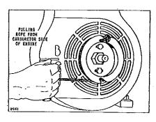
Place knot in pulley notch and wind rope around pulley in a clockwise direction. Pull rope with choke closed to prime the engine. Open choke slightly and repeat operation.
