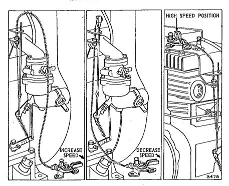
Engine speed is controlled by movement of the control lever. To adjust: Move control lever to HIGH speed position. Loosen screw on swivel. Move wire through swivel until desired operating speed is obtained. Retighten swivel screw, bend loose end of wire around swivel. Cut off excess wire. Be sure to remove or loosen thumb screw on governor control rod.
