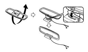
4 Connect the AM loop antenna to the AM terminals on the back of this unit. For best reception, connect an insulated wire (not supplied) in addition to the AM loop antenna. (See "For best AM reception" below.)
