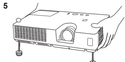
To finely adjust, twist the foot.
