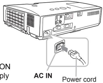
Please remember that when the **DIRECT POWER ON** function activated, the connection of the power supply make the projector turn on.
