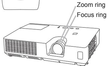
**⚠ CAUTION** ► If you wish to have a blank screen while the projector's lamp is on, use the **BLANK** function. (See the "Operating Guide" in the CD.) Any other method of blocking the projection light, such as attaching something to the lens or placing something in front of the lens, may cause the damage to the projector.
