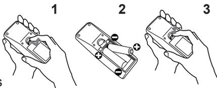
**⚠WARNING** ► Always handle the batteries with care and use them only as directed. Improper use may result in battery explosion, cracking or leakage, which could result in fire, injury and/or pollution of the surrounding environment.
