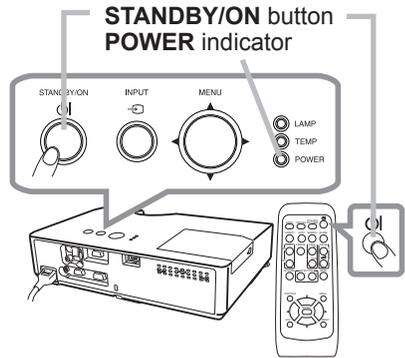
Do not turn the projector on for about 10 minutes or more after turning it off. Also, do not turn the projector off shortly after turning it on. Such operations might cause the lamp to malfunction or shorten the lifetime of some parts including the lamp.
