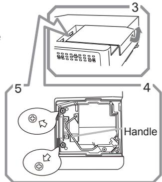
5. Insert the new lamp, and retighten firmly the 2 screws of the lamp that are loosened in the previous process to lock it in place.
