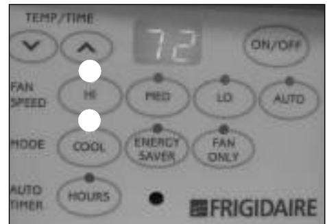
Note: Remember that in this mode, the fan will run continuously while the compressor cycles on and off as needed to maintain the room temperature. (See also, power saver mode, step 6)
