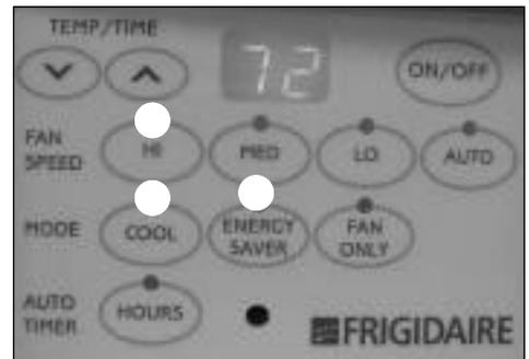
Note: In this mode, when the compressor shuts off, the fan will continue to run for another 3 minutes, then shut off until cooling is needed, as sensed by the room temperature control. During this time, it may come on for 3 minutes to sense whether cooling is needed, then it will go off for 15 minutes. It will continue doing this to sample the room air for as long as necessary.
