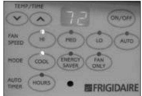
Note: Tap or hold the UP arrow(^) to increase delayed start time by .5 hours (up to 10 hours), then in 1 hour increments up to 24 hours. The control will count down the time remaining until start (8, 7.5, 7, etc.).
