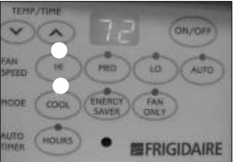
Note: Tap or hold either up(^) or down(v) button until the desired temperature is seen on the screen. This temperature will be automatically maintained anywhere between 60F (15C) and 90F (32C). If you want the display to read the actual room temperature, see step 5.
