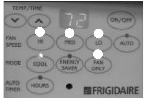
Note: Use this function only when cooling is not desired, such as for room air circulation or to exhaust stale air. (remember to open the vent during this function, but keep it closed during cooling for maximum cooling efficiency.) You can choose any fan speed you prefer. (Note: The "AUTO" setting will not operate in FAN ONLY.)
