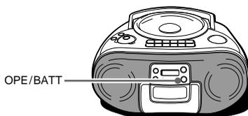
The OPE/BATT indicator lights up while the power is on.
