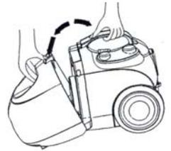
4. Pull up the dust cup filter and shake down and up. Take the dust cup filter out of the dust cup, do not let the dust fall out.
