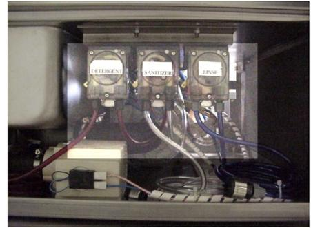
To prime the pumps; you must complete two full wash cycles.
