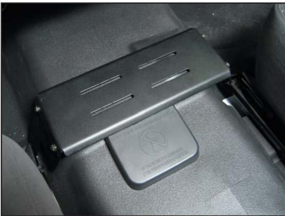
Loosely pre assemble front hump bracket with 1/4" x 3/4" bolts and flat washers, then position it under the OEM front seat brackets.
