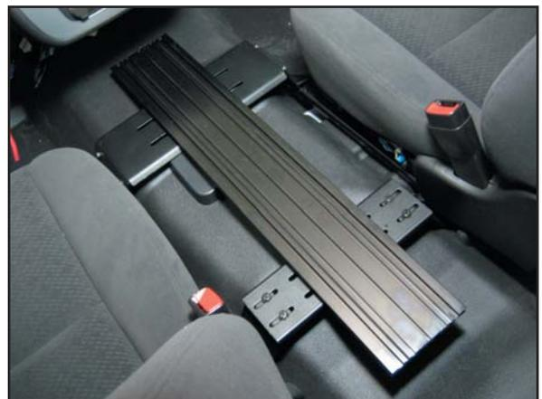
Insert 1/4" x 3/4" bolts into the bottom of Trak.
