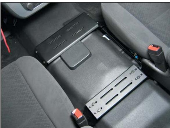
Determine the position of Trak desired and mark location with a pencil on the hump brackets.. Remove the front and rear hump bracket cross support.
