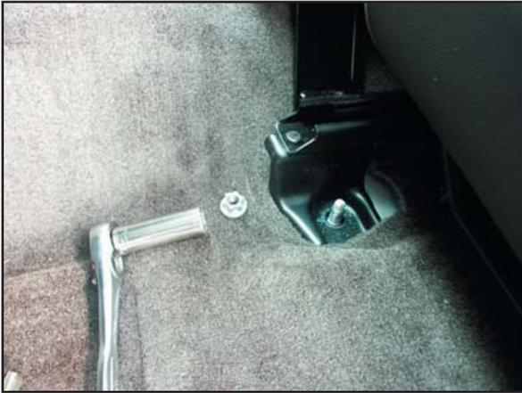
Remove OEM trim panel covering front inner seat bolts on driver and passenger sides.
