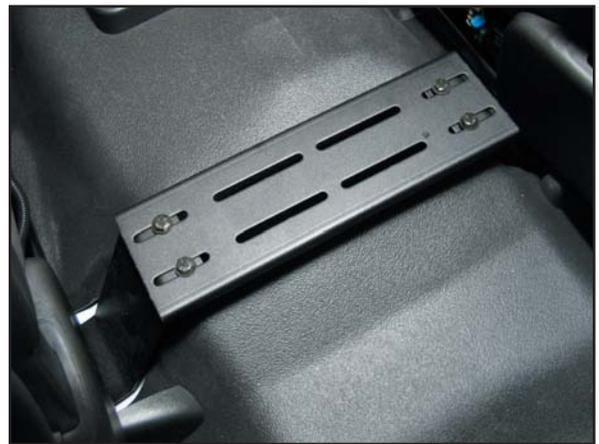
Loosely pre assemble rear hump bracket with 1/4" x 3/4" bolts and flat washers, then position it under the OEM rear seat brackets.
