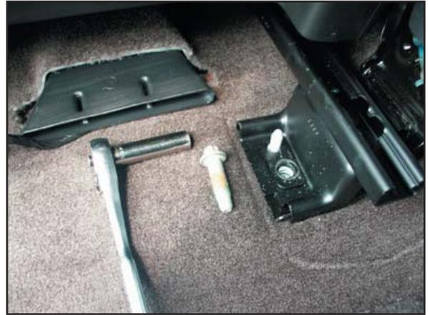
Remove OEM trim panel covering rear inner seat bolts on driver and passenger sides.
