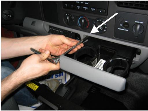
Remove two hex screws on each side of cup holder bracket
