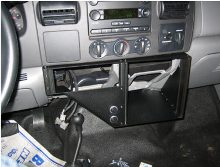
Complete installation of C-VS-0309-F250 console
