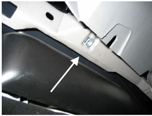
Remove this screw clip to allow a 1/4" bolt to fit into this hole
