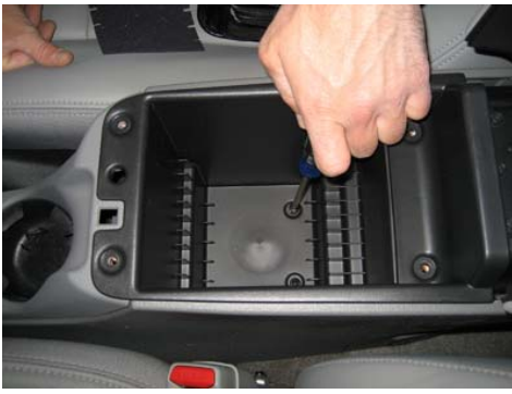
Remove six phillips screws that hold inner storage pocket. Remove storage pocket and arm rest assembly.
