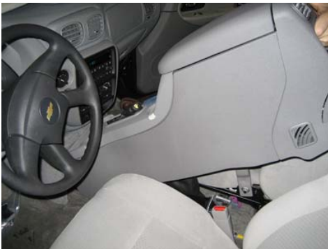
Position shift lever in drive or further back. Remove entire console assembly.
