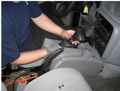
Note: In order to remove console, you must reach up inside the shifter boot and disconnect the traction control plug.
