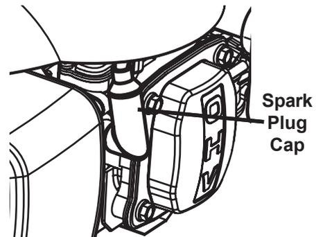
1. Disconnect spark plug cap from end of plug. Clean out debris from around spark plug.
