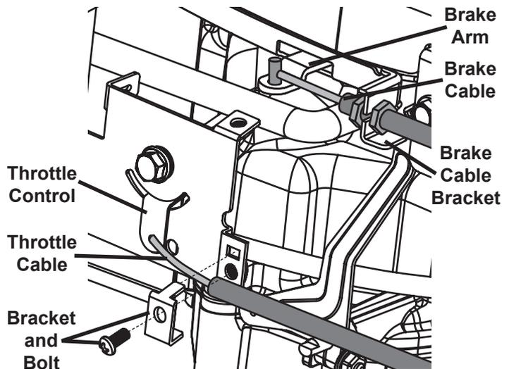
7. Attach the end of the mower's Throttle Cable to the Throttle Control. Use the Bracket and Bolt to secure its sheath in place as shown above.
