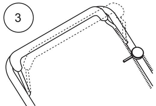
4. Grip the Starter Handle of the Engine loosely and pull it gently until resistance is felt. Allow Cable to retract fully and then pull it quickly. Repeat until the engine starts.
