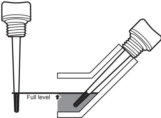
3. Reinsert the Dipstick without threading it in and remove it to check the oil level. The oil level should be up to the full level, the top of the crosshatched area on the dipstick as shown above.
