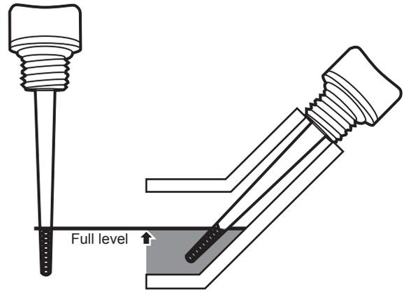
6. Reinsert the Dipstick without threading it in and remove it to check the oil level. The oil level should be up to the full level, the top of the crosshatched area on the dipstick as shown above.
