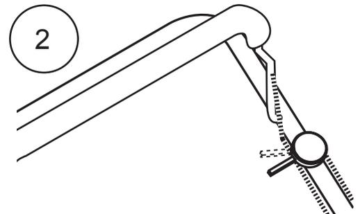
3. Hold the mower's brake handle closed.
