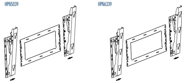
The wall mount bracket is delivered separately. Please tighten the captive screw in the direction of the arrow after assembling the bracket.
