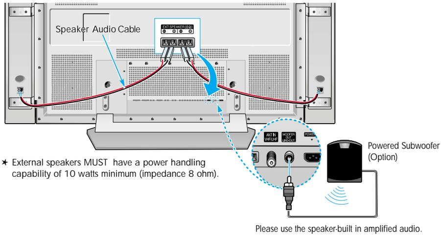
\* External speakers MUST have a power handling capability of 10 watts minimum (impedance 8 ohm).
