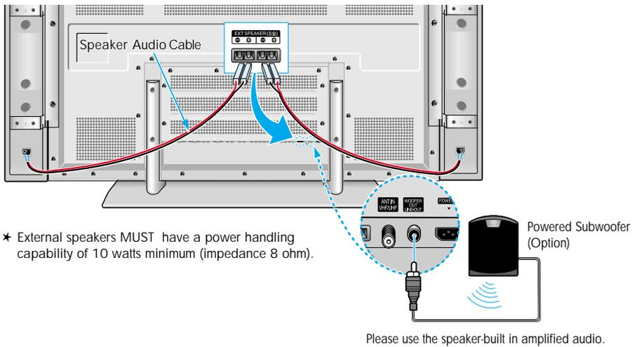
\* External speakers MUST have a power handling capability of 10 watts minimum (impedance 8 ohm).
