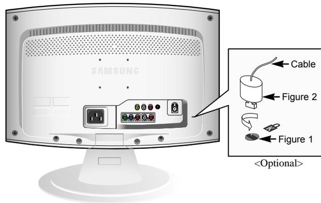
The Kensington lock is a device used to physically fix the system when using it in a public place. The locking device has to be purchased separately. The appearance and locking method may differ from the illustration depending on the manufacturer. Please refer to the manual provided with the Kensington lock for proper use.
