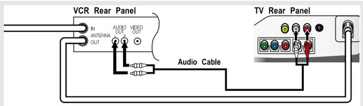
If you have a “mono” (non-stereo) VCR, use the Y-connector (not supplied) to hook up to the left and right audio input jacks of the TV. If your VCR is stereo, you must connect two cables.
