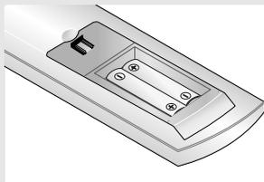
◀ Make sure to match the “+” and “-” ends of the batteries with the diagram inside the compartment.
