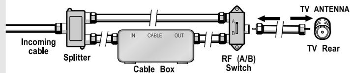
After you've made this connection, set the A/B switch to the "A" position for normal viewing. Set the A/B switch to the "B" position to view scrambled channels. (When you set the A/B switch to "B," you will need to tune your TV to the cable box's output channel, which is usually channel 3 or 4.)
