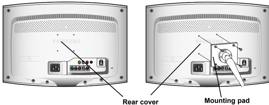
Align the mounting interface pad with the holes in the rear cover mounting pad and secure it with the four screws that come with the arm-type base, wall mount hanger or other bases.
