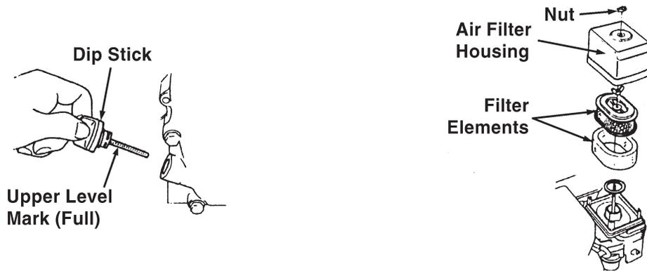
3. Check Air Filter (75) (See illustration above, right). Unscrew Air Filter Housing Nut and remove the Air Filter Housing and Filter Elements. If dirty or dusty, clean (refer to the Maintenance Section).
