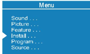
When any item is selected with "△" or "▽" button in the install menu, the selected item will be highlighted on the bottom bar. Changes by pressing "◀" or "▶" button will be result only at highlighted item on the bottom bar.
