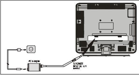
**IMPORTANT:** The TV set is designed to operate on 12 V DC. For this, an adaptor is used which gives 12V DC voltage. Connect this adaptor to a system that supplies 230V AC, 50 Hz.
