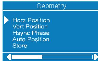
Adjust the required horizontal or vertical position or Hsync Phase by **“◀”**, **“▶”** buttons.
