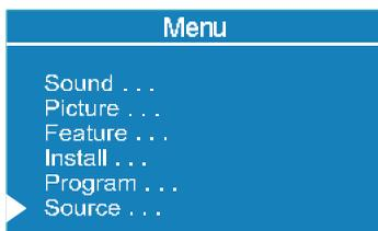
In main menu, firstly use “△” or “▽” button then use “◀” / “▶” or “MODE” button to enter Source menu. In source menu, move the cursor by “△” or “▽” button and then press “MODE” button or “◀” or “▶” buttons when the cursor is on the required item. The selected mode comes automatically on the screen.
