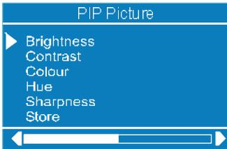
PIP picture is displayed on the screen with **“Ⓢ”** button. By pressing **“MODE”** button, PIP window is selected and border of the PIP window becomes green. PIP position is changed by **“4”** / **“6”** button. There are six different PIP positions. PIP size is decreased by **“8”** button and increased by **“2”** button. Three different PIP size are available.
