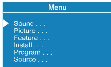
To select a sub-menu use "▲" or "▼" button, and press "◀" or "▶" button or directly press "MODE" button.
