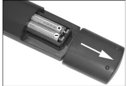
**NOTE:** Remove battery from remote control handset when it is not to be used for a long period. Otherwise it can be damaged due to any leakage of battery.
