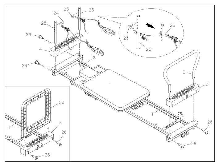
**STEP 4:** Remove the paper covering from the foam tape inside the **FRONT COVER(3)** and **REAR COVER(4)**. Place the **FRONT COVER(3)** over the **FRONT FRAME(1)**. Place the **REAR COVER(4)** over the **REAR FRAME(2)**. Press the covers securely in place.
