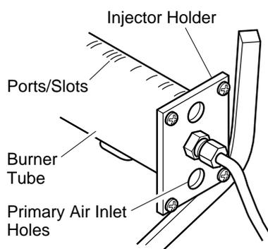
**Figure 43 - Injector Holder On Outlet Burner Tube**
