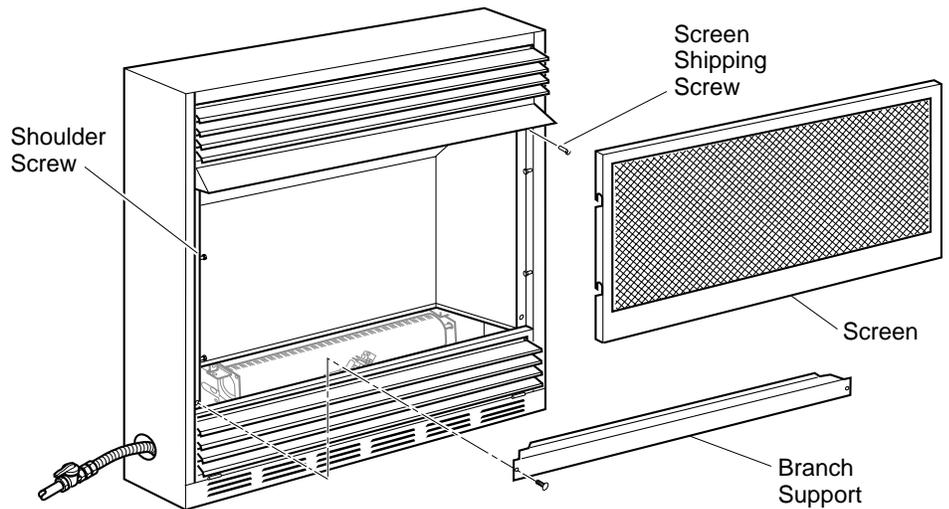
**Figure 23 - Removing Branch Support From Fireplace**
