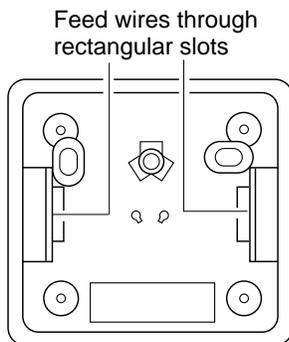
**Figure 32 - Back View of Thermostat Base**
