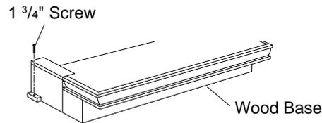
**Figure 13 - Attaching Wood Base to Floor**
