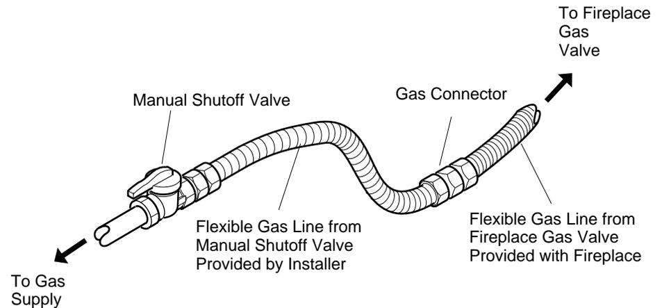
**Figure 24 - Attaching Flexible Gas Lines Together**
