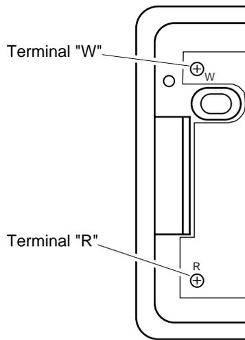
**Figure 33 - Thermostat Base Terminals "W" and "R"**
