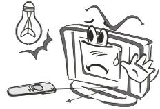
Keep the remote control away from heat sources or humid areas to ensure effective performance of the remote.
