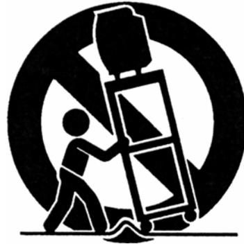
8. Use care when moving the product on a rolling cart. Sudden stops, excessive force and uneven floor surface can cause the product to fall from the cart.
