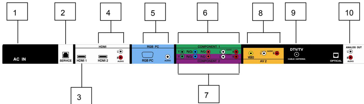
1. **AC IN** – Plug-in the supplied AC Power Cord here.
