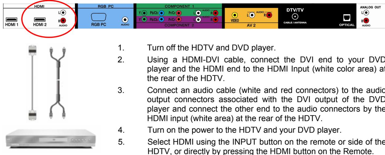
The image shows the rear panel of the VIZIO HDTV with various input ports. The HDMI 2 port is circled in red. Below the panel is a photograph of the HDTV with an HDMI-DVI cable and an audio cable plugged into the HDMI 2 port.
