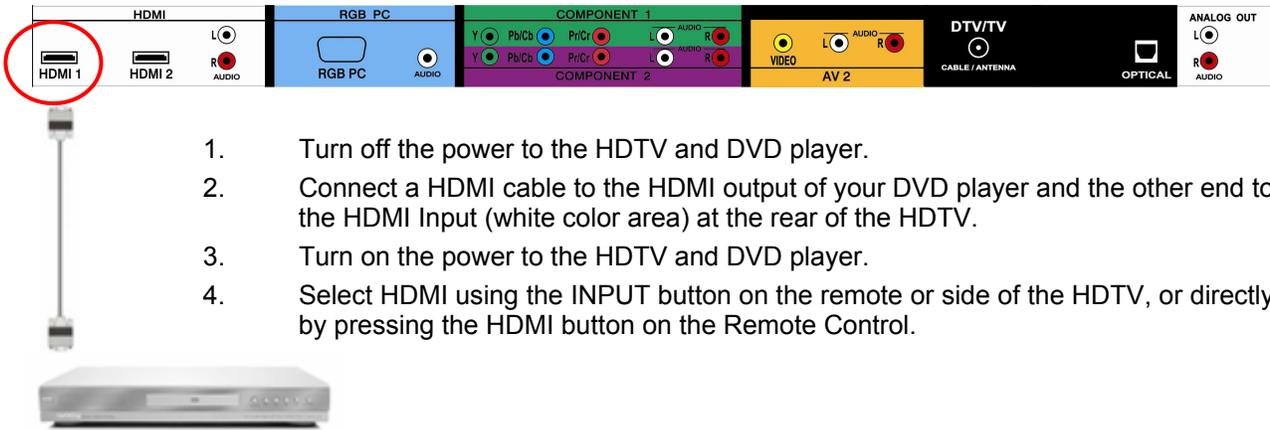
The image shows the rear panel of the VIZIO HDTV with various input ports. The HDMI 1 port is circled in red. Below the panel is a photograph of the HDTV with an HDMI cable plugged into the HDMI 1 port.
