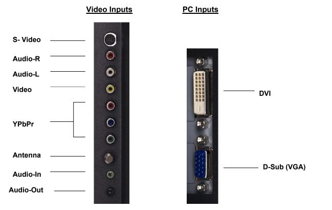
**Note:** The Audio-L and Audio-R (Audio L/R) inputs are shared between YPbPr, S-Video, and Video source input connectors.
