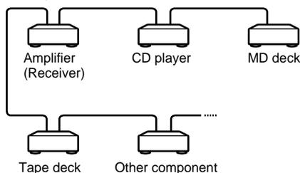
In the CONTROL A1II control system, the control signals flow both ways, so there is no distinction of IN and OUT jacks. If a component has more than one CONTROL A1II jack, you can use either one, or connect different components to each jack.
