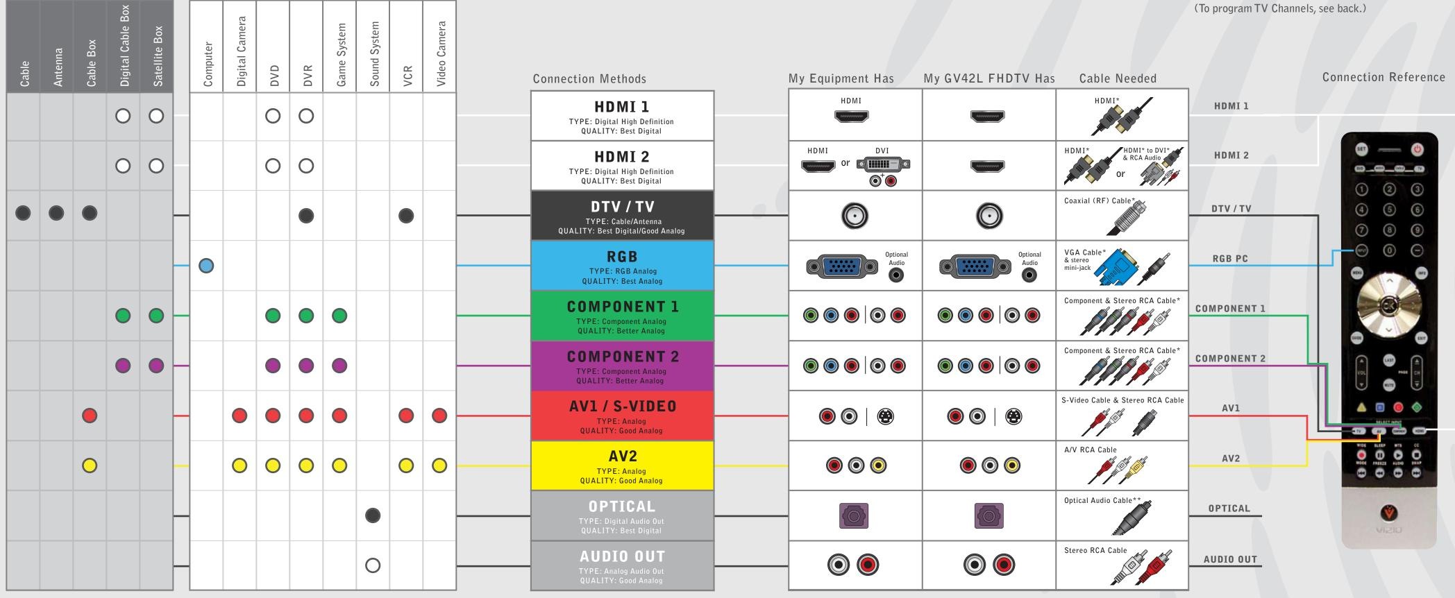
To Use This Chart: Write your equipment or signal source into the squares corresponding to your connection method.
