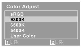
**sRGB-**This is quickly becoming the industry standard for color management, with support being included in many of the latest applications. Enabling this setting allows the LCD display to more accurately display colors the way they were originally intended. Enabling the sRGB setting will cause the Contrast and Brightness adjustments to be disabled.
