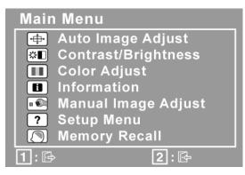
**NOTE:** All OSD menus and adjustment screens disappear automatically after about 15 seconds. This is adjustable through the OSD timeout setting in the setup menu.
